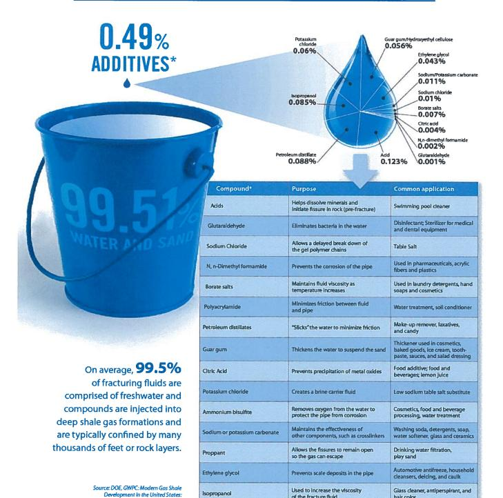
The specific compounds used in a given fracturing operation will vary depending on source water quality and site, and specific characteristics of the target formation. The compounds listed above are representative of the major material components used in the hydraulic fracturing of natural gas shales. Compositions are approximate.
